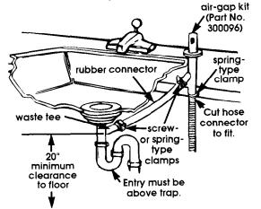
Drain hose to air gap to disposer.
