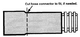
If connecting drain hose to an air gap or waste tee, cut end of drain hose as shown.
