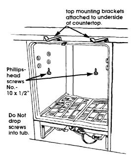
**12.** Open dishwasher door and remove all shipping materials. Remove bottom rack. Place a newspaper or large sheet of paper over bottom of dishwasher to protect the pump area when securing dishwasher to countertop.
