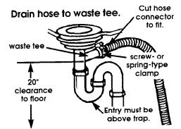
If local plumbing codes permit, dishwasher drain hose may be connected directly to waste tee\*. The waste tee connection MUST be made ahead of the trap and a minimum of 20" above the floor.
