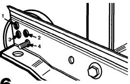
• Measure height of cabinet opening from the front edge of the underside of cabinet opening to floor. Check chart for that height opening. Put the wheels in the required position. The dishwasher should be installed as level as possible from front to back.
