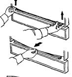
**3.** Insert one side of door panel(s), with desired color facing out, into one side of door frame.
