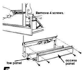
■ Remove the 4 screws attaching access panel and toe panel to dishwasher using a 1/4" hex socket, nut driver or Phillips screwdriver. Remove access panel and toe panel.
