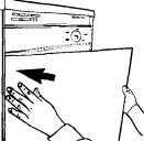
**4** Bow door panel(s) and insert other side of door panel(s) into door frame.
