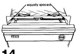
and check for equal spacing between inner door and tub sides. If necessary, loosen screws that fasten dishwasher to countertop and shift tub. Tighten screws.
