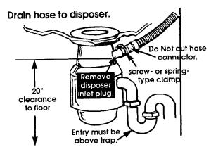
If local plumbing codes permit, dishwasher drain hose may be connected directly to disposer. Most disposers have 7/8" connectors or special connectors are available at plumbing supply houses.
