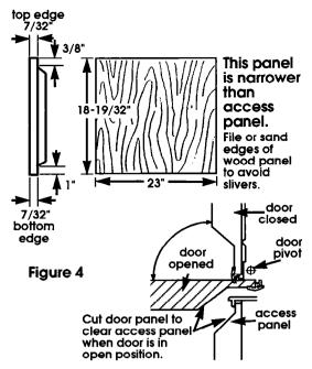
Heavy-duty door springs must be used if custom door panel weighs more than 4 pounds. Heavy-duty Door Springs Kit, Part No. 4318050, is available from your dealer or parts supplier. Maximum door weight is 8 pounds.
