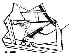
**16** Check door for proper operation. Door should close easily without slamming and open with its own weight. If necessary, close door and adjust both door springs by moving spring ends to different holes in base.
