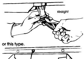
Cut a 1-1/2" maximum hole for power supply cord or a 3/4" minimum hole for direct wiring in the cabinet or floor for the electrical wiring to pass through. If this hole is cut in a wood cabinet, sand the hole until it is smooth. If the hole is cut in a metal cabinet, the hole **must** be covered by a grommet (Part No. 302797), available from your dealer or parts supplier.
