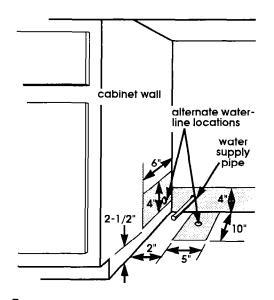
■ Rough in water line to the dishwasher cabinet opening using one of the routing methods shown. Cut 1/2" or larger hole in cabinet wall for water line.
