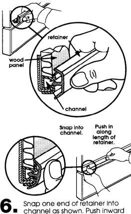
channel as shown. Push inward while sliding thumb along full length of retainer.
