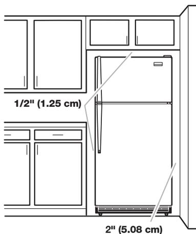
To ensure proper ventilation for your refrigerator, allow for 1/2" (1.25 cm) space on each side and at the top.
