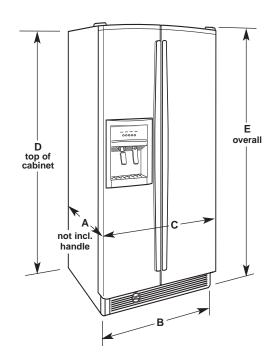
Dimensions "D" and "E" include rollers extended 3/4".
