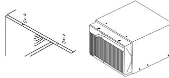
Your unit may come with internal packaging. THIS PACKAGING MUST BE REMOVED PRIOR TO INSTALLING THE AIR CONDITIONER BACK INTO THE CABINET. (See FIG. 5)...
