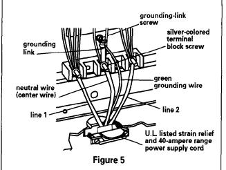
Use this method for mobile homes and whenever four-wire installation is required.
