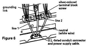
Use this method ONLY if local codes PERMIT connecting cabinet-grounding conductor to neutral wire of power supply cable.
