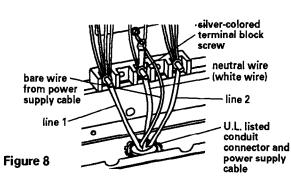
Use this method for mobile homes and whenever four-wire installation is required.
