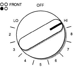
Check the operation of the cooktop elements: Push in and turn each surface unit control knob to "HI" position. Check the operation of the cooktop elements and indicator lights.
