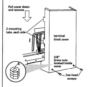
Remove the terminal block cover screws ■ located on the back of range. Pull cover down and towards you to remove cover from range.
