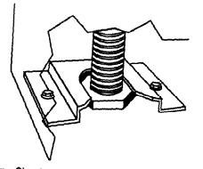
9 Check that rear leveling leg is engaged in anti-tip bracket.
