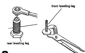
Remove storage drawer. Use a 3/8\* drive ratchet to lower rear leveling legs one-half turn. Use channel lock pliers to lower front leveling legs one-half turn.
