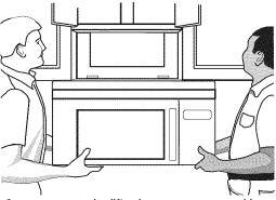
3. Using 2 or more people, lift microwave oven and hang it on support tabs at the bottom of mounting plate.
