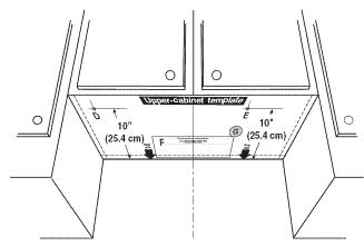
5. Cut the 1½" (3.8 cm) diameter hole at the circular shaded area "G" on the template. This hole is for the power supply cord.
