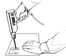
To mount the anti-tip bracket to a concrete or ceramic floor, use a 3/16" (4.8 mm) masonry drill bit to drill 2 holes at the positions marked on the bracket template. Remove the template from the floor.
