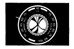
4. To change the setting at any time, turn the Cycle Control Knob either way to point to a new time setting.
