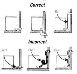
▲ WARNING — The following are specific requirements for proper and safe operation of your dryer. Failure to follow these instructions can create excessive drying times and fire hazards.
