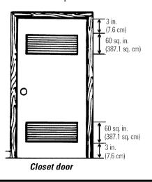
Allow the following clearances for ease of installation:
