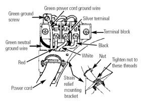
**A WARNING:** Do not make a sharp bend or crimp wiring/conductor at the connections.
