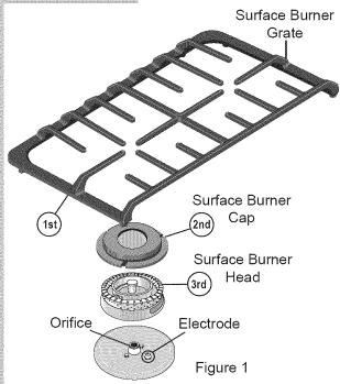
The Grates, Burner Caps and the Large 18k Burner Head should be routinely cleaned. Keeping the burner ports clean will prevent improper ignition and an uneven flame. If needed, the fixed burners should be cleaned in place with an humid cloth (do not spraw water on them).
