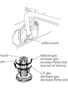
**D** Broil burner: Use 1/2" combination wrench to turn the orifice hood down snug onto pin (approximately 2 to 2-1/2 turns). Do not overtighten. The burner flame cannot be properly adjusted if this conversion is not made.
