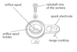
Locate the L.P. gas orifice spud on the spud card on the back
