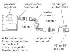
**10** Use 5/16" combination wrench and channel lock pliers to attach the flexible connector to the adapters. Check that connector is not kinked.
