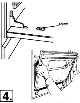
Close lower oven door to the broil position. Grasp the sides of the oven door and pull the door up and out of the hinge slots to remove. Set door aside.
