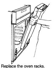
Replace the oven door by partially fitting the door hinges into the hinge slots. Pull door slightly toward you; then slide door completely in place. Reinstall the two oven-door screws (if required for your oven door). If door does not close, you have not pushed hinges completely into frame. Repeat for lower oven door.
