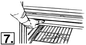
Remove and discard shipping base. Lift oven up into cabinet cutout using the oven opening as an area to grip.
