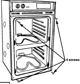
Center oven into cabinet cutout. Use four screws through the mounting holes in the front frame of the oven to secure the oven to the cabinet. Do Not overtighten screws.
