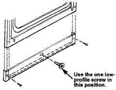
Install the lower vent grille using the three screws provided.
