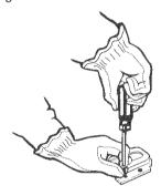
**6** ■ Use the anti-tip bracket template to install the anti-tip bracket.
