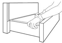
Pull drawer open to first stop position. Lift front of drawer to clear white wheels in drawer guides. Remove drawer and set it aside on a protected surface.
