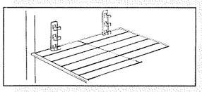
Three position adjustable shelf can be moved to any one of three positions for larger or smaller packages.
