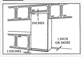
Allow three inches of air space on all sides of the freezer.
