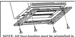
NOTE: All four-levelers must be reinstalled in bottom of cabinet after skids are removed.
