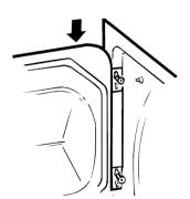
**3** Rotate the door 180°. Insert it on the opposite side of the opening by moving the door **IN** and **DOWN** until the top hinge and the bottom hinge are resting on the top screws inserted in step 1.
