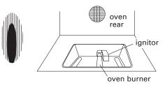
26 If the oven flame needs to be adjusted, locate the air shutter near the center rear of range. Loosen the locking screw and rotate the air shutter until the proper flame appears. Tighten locking screw.
