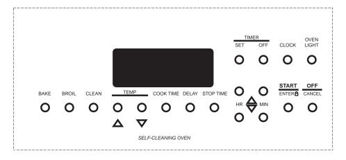
**24** • Check the operation of the oven burner. Push the "BAKE" pad and "Pre°F" will appear in the temperature display. Press the "START/ENTER" pad. A preheat time will count down. The oven burner should light in 50 to 60 seconds. This delay is normal. The oven safety valve requires a certain time before it will open and allow gas to flow.
