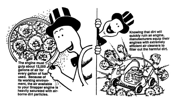
As the dirt particles are stopped. they build up and begin to clog the outside of the filter. This reduces the amount of air available to the engine and causes an over-rich fuel mixture which resuits in the following adverse effects:
