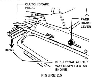
**5.** Choke engine for cold starting by moving engine speed control to "CHOKE" position. **NOTE:** Some models are equipped with a separate choke control, located on the dash of the tractor. Pull the control "OUT" to choke position to start a cold engine. Little or no choking will be needed when restarting a warm engine. Insert key in switch. Turn key to "START" position to crank engine and hold until engine starts, then release key to "RUN" position. See Figure 2.6.
