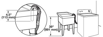
Minimum capacity: 20 gal. (76 L). Top of laundry tub must be at least 39" (991 mm) above floor; install no higher than 96" (2.4 m) from bottom of washer.
