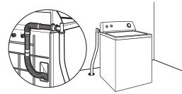
Floor drain system requires a Siphon Break Kit and additional drain hose that may be purchased separately. See "Tools and Parts". Minimum siphon break: 28" (711 mm) from bottom of washer. (Additional hoses might be needed.)
