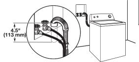
See requirements for floor standpipe drain system.
