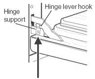
Lock engaged for door removal Figure 1
