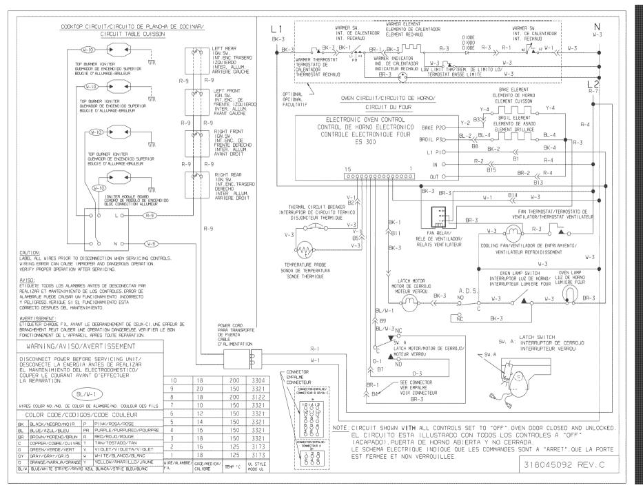
WIRING DIAGRAM -SCHÉMADE
