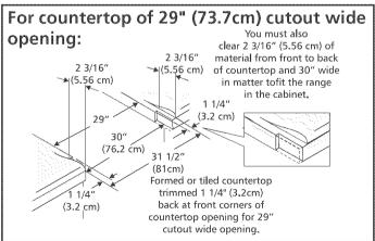
• Countertop must be level. Place a level on the countertop, first side to side, then front to back. If the countertop is not level, the range will not be level. The oven must be level for satisfactory baking results. Cooktop sides of range fit over edges of countertop opening.
