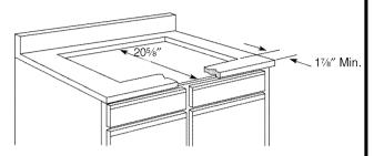
A 1/2" wide flat area is required around the edge of opening for support of the unit. The cooktop unit must be level and sit squarely into countertop opening.
