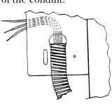
Place the clamp over the conduit. Make sure the bushing is fully seated against the stop tab in the clamp.
