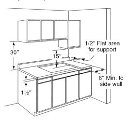
Avoid placing cabinets above the cooktop unit, if possible, in order to reduce the hazards caused by reaching over heated surface units. If cabinets are placed over the cooktop, the risks can be reduced by installing a range hood that projects horizontally a minimum of 5" beyond the bottom of the cabinets.
