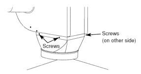
to connect to 5" round standard ductwork. Install the transition duct to the blower outlet with four (4) sheet metal screws. Secure all joints with duct tape to assure an airtight seal.
