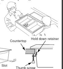
Secure cooktop to the counter using the hold down retainers and thumb screws shipped with the unit (one on each side).
