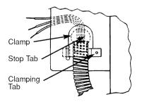
Tighten the clamping screw until the clamping tab is fully seated against the wire compartment.
