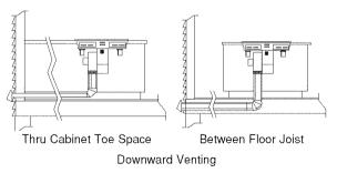
Install ductwork, making male-female connections in direction of airflow as shown. Secure all joints with sheet metal screws and duct tape to assure airtight seal.
