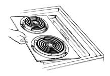
2. Slide the module toward the outlet in the side of the cooktop until the plug is pushed all the way in.
