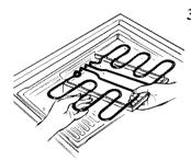
3. Make sure all controls are turned to OFF. Hold the heating element with the plug facing the side of the cooktop and level with the surface. Insert the plug into the cooktop outlet as far as it will go. (Do not force.) The heating element support should rest on the ledge of the reflector pan.
