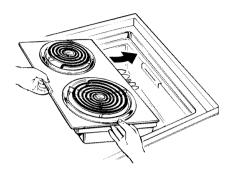
1. Be sure the controls are turned to OFF. To install the module. position the plug to the outside wall of the cooktop.
