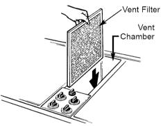
Remove and replace the filter diagonally through the vent opening.
