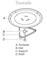
The turntable can rotate in either direction to help cook food more evenly. Do not operate the oven without the turntable in place. See "Assistance or Service" to reorder any of the parts.
