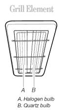
The oven uses a 1,000-watt halogen bulb with a 500-watt quartz bulb to serve as the grill element for various cooking functions.
