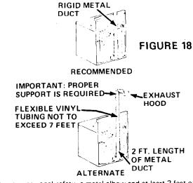
For your personal safety, a metal elbow and at least 2 feet of metal duct must be used at the outlet of the dryer. This reduces the possibility of lint blocking the exhaust system and minimizes the potential of a fire hazard. The 2 feet of metal duct also helps make any service that may be needed easier and prevents crushing the flexible duct when the dryer is moved to its final operating location.
