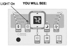
**Note:** This feature is a reminder to clean the Air Filter (See Care and Cleaning) for more efficient operation and cooling. The LED (light) will illuminate after 250 hours of operation. To reset after cleaning the filter, press the "Check Filter" button and the light will go off.
