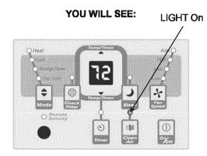
Note: When this feature is "ON", the electronic air purifier is energized to remove pollen and impurities from the air. To cancel this feature,
