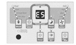
If the display reads"ES", a sensor has failed.
