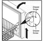
**4** Close drawer and recheck the seal on the gasket (A). Open the drawer grabbing by the sides in the center (B). Be careful not to rotate the drawer.
