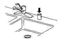
The drain air gap is usually located on top of the sink or countertop near the dishwasher. To order a drain air gap contact your local dealer, or in the U.S.A., call the Consumer Assistance Center at 1-800-422-1230 and ask for Part Number 300096.
