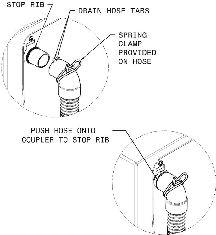
3. Using pliers, squeeze the ears of the spring clamp and position the clamp so the clamp ears align with and contact the tabs on the drain hose. This assures proper location of the clamp to prevent leaks.
