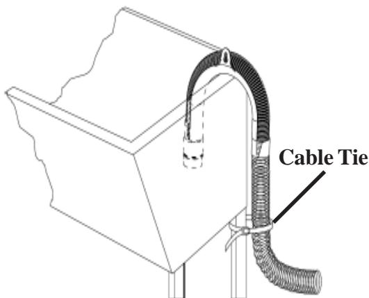
5. Place the hook end of the drain hose in the drain opening. Secure the drain hose with the cable tie (provided in the enclosure package) to the standpipe, inlet hose, laundry tub, etc. so the hose does not pull out from the force of the water.
