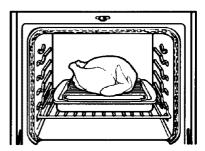
• Use the convection roasting rack on the broiler pan (both included with your range). (The convection roasting rack rests on the broiler pan, not inside it.) The long side of the rack should be parallel with the oven door for best heat distribution and airflow.
