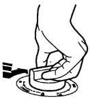
• Push in and turn the control knob to the right (clockwise) to the desired setting in the area marked "DUAL".
