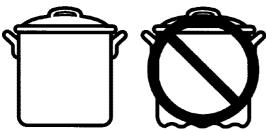
NOTE: For best results and greater energy efficiency, use only flat-bottomed cookware that makes good contact with the surface units. Cookware with rounded, warped, ribbed (such as some porcelain enamelware), or dented bottoms could cause uneven heating and poor cooking results.
