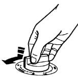
• **Push in and turn** the control knob to the left (counterclockwise) to the desired setting in the area marked "SINGLE".
