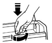
To remove and replace the starter, first remove light tube. Push starter in and turn approximately 90° counterclockwise. Pull starter out of recessed area. You can find replacement starters at stores that sell fluorescent light tubes.
