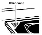
Hot air and moisture escape from the oven through a vent in the left rear corner of the cooktop. **Do not block the vent by using large pans or covers.** Poor baking/roasting can result.
