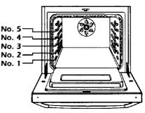
Your oven has three straight racks and five rack positions. Rack position 5 is the highest position, or farthest from the bottom of the oven. Rack position 1 is the lowest position, or closest to the bottom of the oven.
