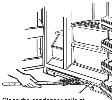
Clean the condenser coils at least once a year.
