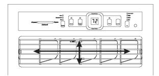
The 4-Way air directional louvers allow you to direct air flow up or down, left or right throughout the room as needed.
