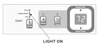
**NOTE**: In this mode, the fan will continue to run for 3 minutes after the compressor shuts off. The fan then cycles on for 2 minutes at 10 minute intervals until the room temperature is above the set temperature, at which time the compressor turns back on and cooling starts.
