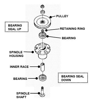
**5.** Thoroughly clean all parts removing all old contaminated grease.
