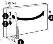
**3** Remove the handle fastener with a Phillips
