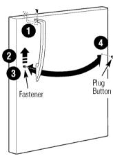
**After removing the handle:** Move the small plug buttons from the top right side of the door top and insert them into the holes on the opposite side.
