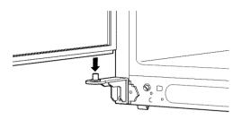
Straighten the door and line it up with the center hinge bracket.
