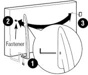
2 Remove the handle fastener with a Phillips
