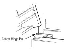
Lift the top hinge so the pin fits into the door socket. Support the door on the handle side and make sure the door is straight and the gap between the doors is even across the front. While holding the door in place, tighten the top hinge screws.
