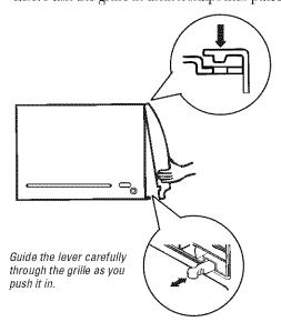
Lift the inlet grille and secure the front frame with a type A screw through the front grille.
