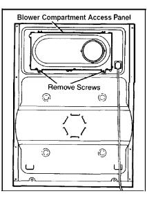
With dryer unplugged, remove two Phillips-head screws at bottom of blower compartment access panel. Tip bottom of panel out until clips slip out. To replace, slip top of panel up until clips are secured. Press bottom of panel in and replace screws.
