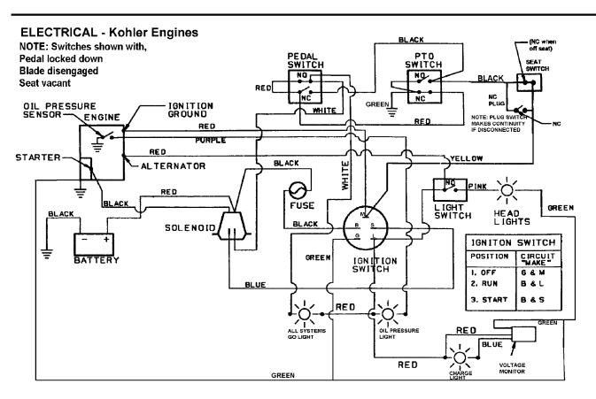
SCHEMATIC – WIRING HARNESS P.N. 2-4815 LT15OHGKV
