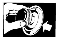
B. Restart the washer by pulling out the Control Knob.
