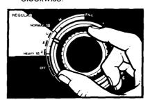
**B.** To select wash water temperature, stop on the area in the selected cycle marked H (hot), W (warm) or C (cold).
