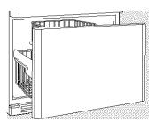
**On drawer models:** The lower basket slides out when the drawer is opened to provide easy access to foods stored in this basket. The upper basket may be pushed back to further improve access to the lower basket.
