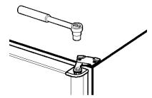
Lift the hinge straight up to free the hinge pin from the socket in the top of the door.
