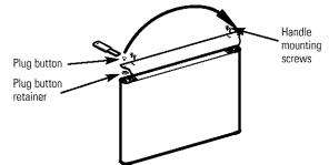
Remove the plug button and transfer it to the opposite side.
