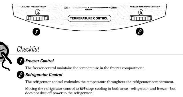
After changing the controls, allow 24 hours for the refrigerator to reach the temperature you have set.
