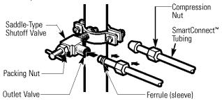
Check if the shutoff valve is closed before advancing to the next step.
