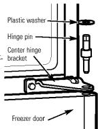
Lift the door straight up to free its bottom socket from the pin in the bottom hinge bracket.
