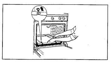
To replace: Insert the tabs into the slots on the back oven wall. Lower into place. Slide two screws forward and tighten. Be sure bottom is fitted into slots and screws are tight. If not correctly replaced, oven bottom may become warped and cooking results will be affected.
