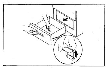
**To replace:** Slide grooves at top of drawer onto guide rails at sides of broiler compartment and push drawer in to close.
