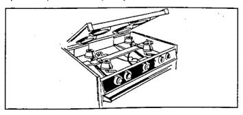
**To replace:** Insert the two pins on the back of the cooktop into the holes in the backguard. Lower the top into place applying pressure at the front edges to secure top to the range.
