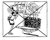
Do not obstruct the flow of combustion and ventilation air by blocking the oven vent or air intakes. Restriction of air flow to the burner prevents proper performance and increases carbon monoxide emission to unsafe levels.
