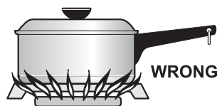
Improper Flame Size
