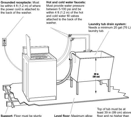
enough to support a total weight of 315 lbs (143 kg) (including washer, water, and load weight).
