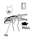
**STEP 3.** Cut the shipping strap about 16 in (40 cm) from plug end. Look for the words "CUT HERE." Discard end with the cotter pins. **Slide remainder of shipping strap from the electrical plug.** You will use this to secure the drain hose.
