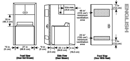
\*Additional clearance for wall, door and floor moldings may be required. To reduce the transfer of washer sounds, a clearance of 1 in (2.5 cm) on the sides of the washer is suggested.
