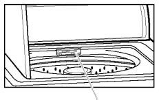
Model and Serial Number Plate Use the space below to record the model number and serial number of your new Kenmore washer.
