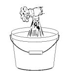
**STEP 2.** Attach the hose with the red coupling to the hot water faucet. Screw on coupling by hand. Make an additional two-thirds turn with pliers to tighten coupling. DO NOT OVERTIGHTEN; this could damage the coupling.
