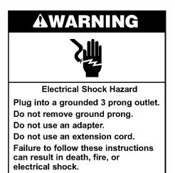
This washer is equipped with a power supply cord having a 3-prong grounding plug. To minimize possible shock hazard, you must plug the power supply cord into a mating 3-prong grounding-type wall receptacle, grounded in accordance with National Electrical Code, ANSI/NFPA 70latest edition and all local codes and ordinances.
