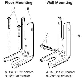
5. Using a Phillips screwdriver, mount anti-tip bracket to the wall or floor with the two #12 x 15/8" screws provided.
