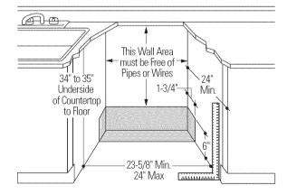
• The rough cabinet opening must be at least 24" deep, 23-5/8" min. to 24" wide. The height should be 34" min. and 35" max.
