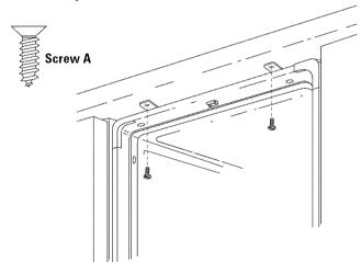
IMPORTANT: To avoid damage to your dishwasher, drive screws straight and flush. Protruding screw heads may scratch the top of the escutcheon or door and can interfere with door closing.
