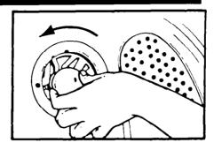
2. Remove the light bulb by turning it counterclockwise.
