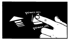
Move the POWER SWITCH **up**. You will have 8 seconds to touch a FABRIC-TEMP Selector.
