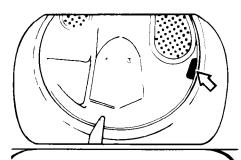
A sensor on the back of the dryer drum "feels" the amount of moisture in the load. When the dryness you have selected is reached, the dryer automatically shuts off.
