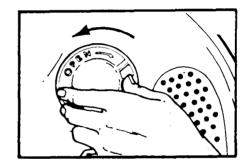
Replace the light bulb cover and lock it in place by turning counterclockwise.
