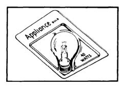
3. Replace the bulb only with a 40-watt appliance bulb from most hardware, grocery or variety stores.
