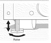
Adjustable Front Roller (some models) Stationary Front Roller with Leveling Screw (some models)
