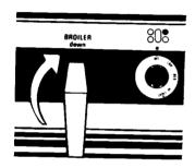
The handle located to the right of the Broiler/Griddle raises and lowers the Broiler Platter, moving it closer or further away from the burner depending upon the foods you are broiling.
