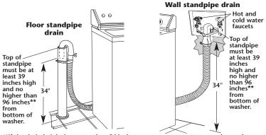
\*\*If the drain height is greater than 96 inches, a sump pump system must be used.
