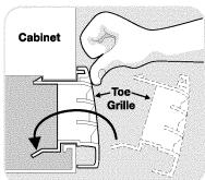
3. Starting from left side of toe grille, press in on first top tab using your thumb and push toe grille forward until it snaps in place. Continue this process until all tabs are snapped in place and toe grille is secured to refrigerator.
