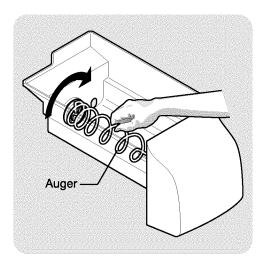
**IMPORTANT:** When removing or replacing the ice bin, do not rotate the auger in the ice bin. If the auger is accidentally turned, you must realign the auger by turning it in 90° turns until the ice bin fits into place with the drive mechanism.
