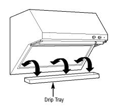
Baffle grease filters and drip trays (on some models) Some models have reusable metal grease baffles and drip trays.
