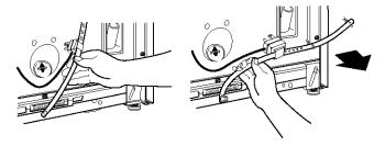
2. Pull firmly to remove the end of the shipping strap that remains pinned to the back of the washer. This will release the rear self-leveling feet.
