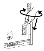
5. Place clamp over area marked "CLAMP." Release clamp.
