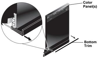
2. Grasp top and bottom of panels and bow slightly until they are clear of trim. DO NOT REMOVE SPACER.
